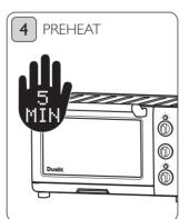
Ensure the oven door is closed. Preheat the oven for five minutes. The temperature light will turn off when the set temperature is reached. The oven is now ready for cooking.
